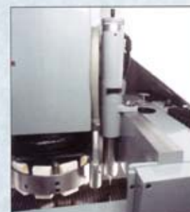
Rilevatore di livello RTS 15 Diamond tipped probe RTS 15 for stock removal control and automatic wheel wear compensation
