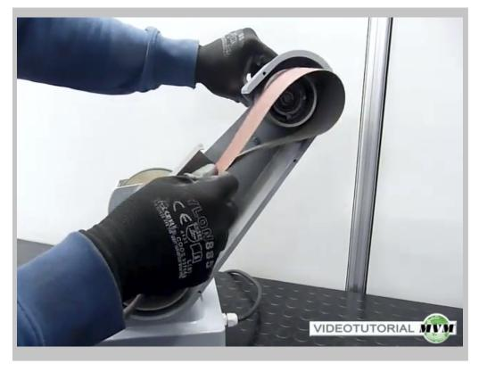
Turn the lever, insert the new abrasive paper band and then release the lever to tension the belt.
