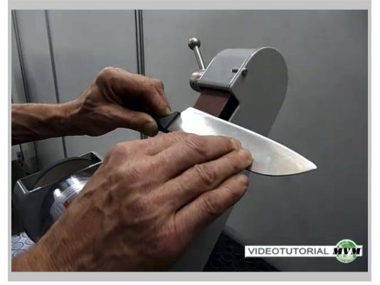
With a slight pressure pass the knife edge across the abrasive paper in the upper flexible zone to sharpen the bevel angle on both sides. The abrasive paper tends to adapt to the bevel angle of the knife.
