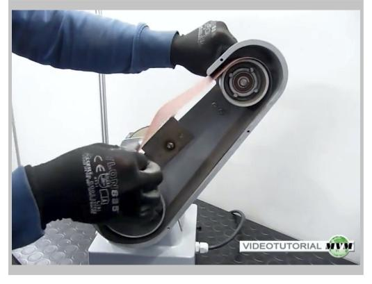
Remove the abrasive paper and then release the lever.
