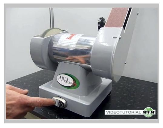
Press the ON button to start the machine.
