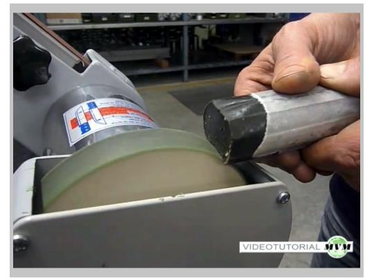
Apply silicone paste to the buffing wheel with a slight pressure of the stick of paste (supplied).
