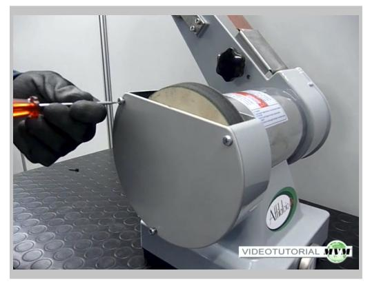
Finally, reposition the cover and tighten the 4 screws.
