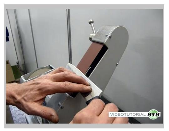
With a slight pressure pass the knife across the abrasive paper in the lower rigid zone to sharpen the cutting angle on both sides. The cutting angle is determined from the manual position of the knife.
