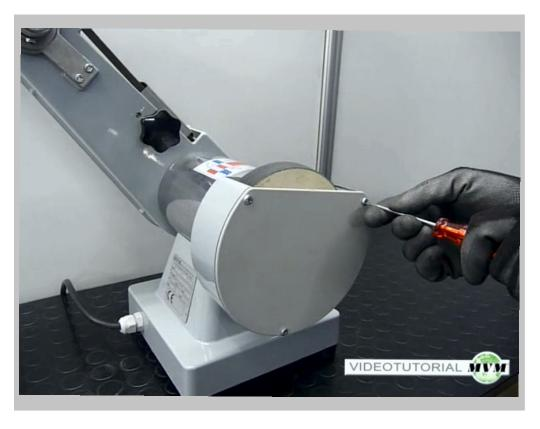
Remove the 4 screws and remove the cover.
