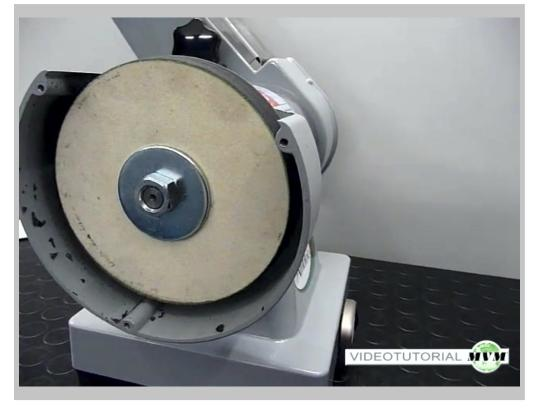
Unscrew the nut and remove the buffing wheel to be replaced. Mount the new wheel and tighten the nut.
