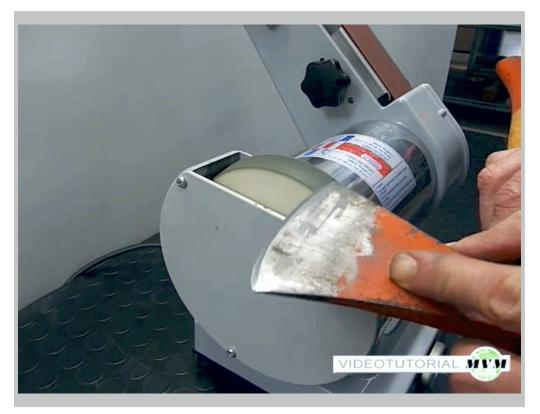
With a slight pressure pass the knife across the buffing wheel to polish the knife on both sides.
