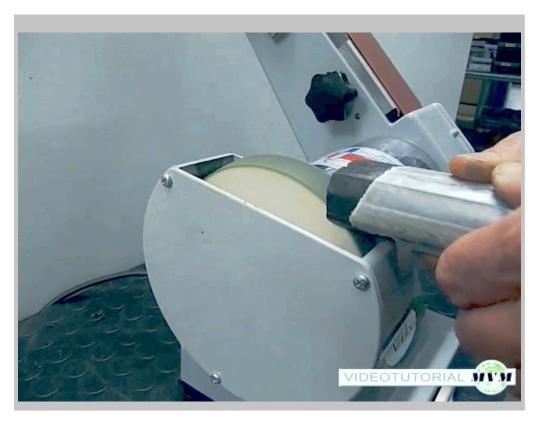
Apply silicone paste to the buffing wheel with a slight pressure of the stick of paste (supplied).
