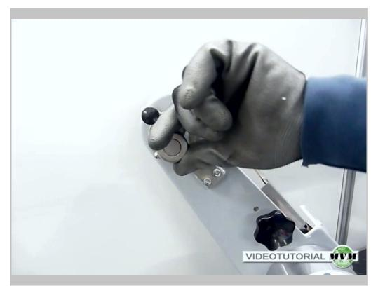
Turn the lever to loosen the belt.
