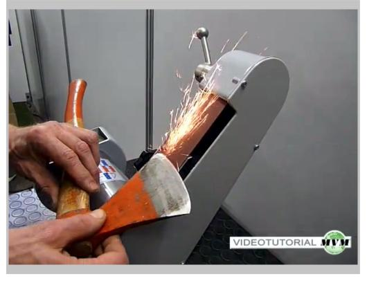
With a slight pressure pass the knife edge across the abrasive paper in the upper zone flexible to sharpen the bevel angle on both sides.
