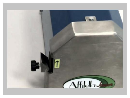
Fix the two 45 ° angle references on the grinding wheel housing, one on the right and one on the left of the grinding wheel.
