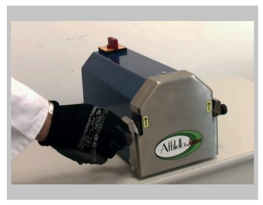
Fix the two 30° angle references on the grinding wheel housing, one on the right and one on the left of the grinding wheel.
