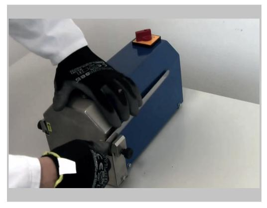
Turn the switch to position 2, place the blade of the knife on the right reference edge in contact with the grinding wheel and make 2-3 sharpening passes back and forth.
