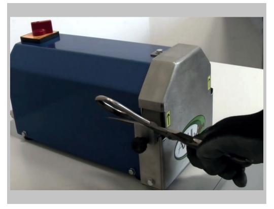
Place each blade of the scissors against the reference inclined at 45° and make contact with the grinding wheel. Then make 2-3 sharpening passes back and forth across the grinding wheel for each blade.
