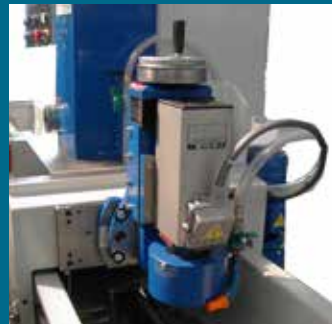
Testa superfinitura TSF Superfinish head Zusätzlich Feinschleifkopf
