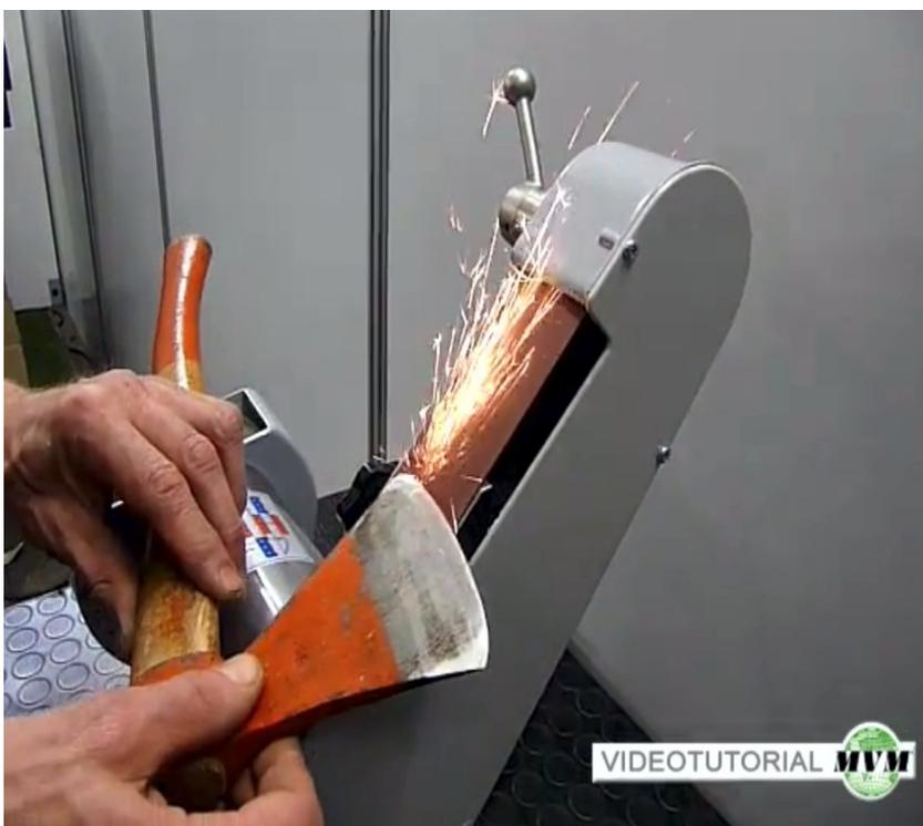
With a slight pressure pass the knife edge across the abrasive paper in the upper zone flexible to sharpen the bevel angle on both sides. The abrasive tape paper tends to adapt the bevel angle of the blade. In the lower rigid zone sharpen the cutting angle on both sides. The cutting angle is determined from the manual position of the blade.
