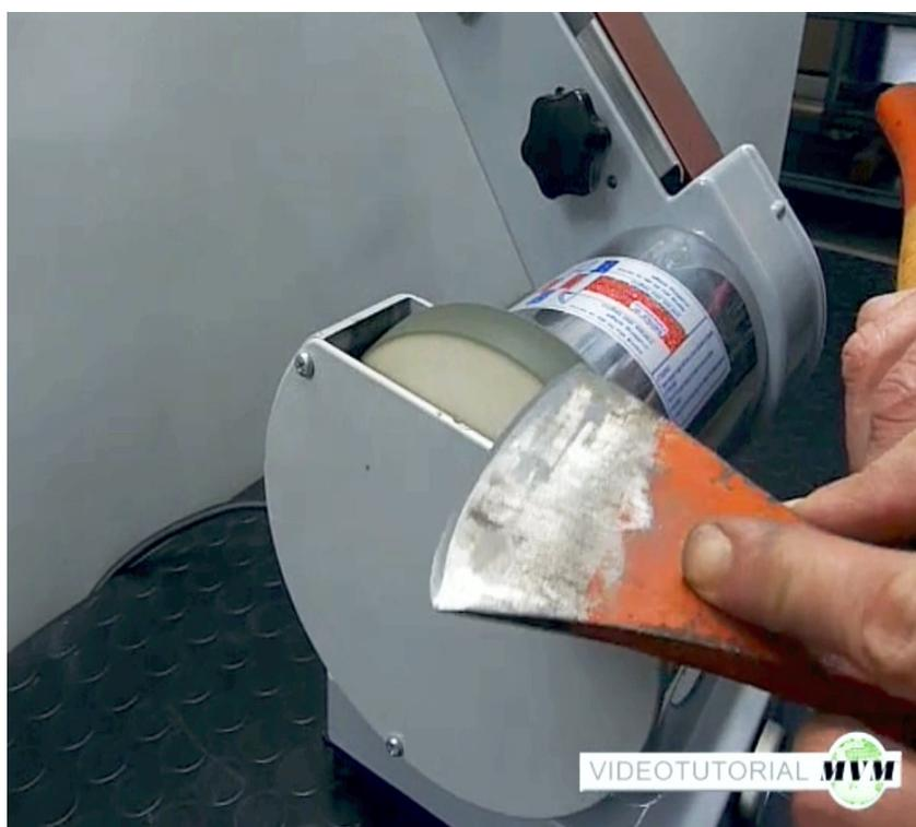
With a slight pressure pass the knife across the buffing wheel to polish the knife on both sides.
