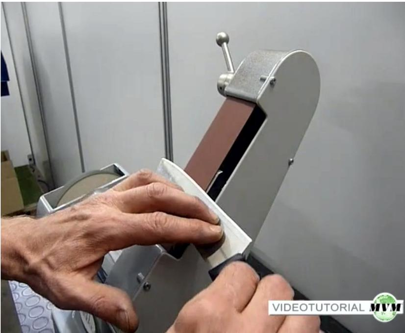
With a slight pressure pass the knife across the abrasive paper in the lower rigid zone to sharpen the cutting angle on both sides. The cutting angle is determined from the manual position of the knife.
