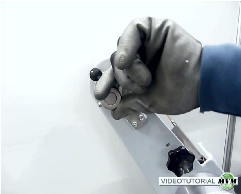
Turn the lever to loosen the belt.
