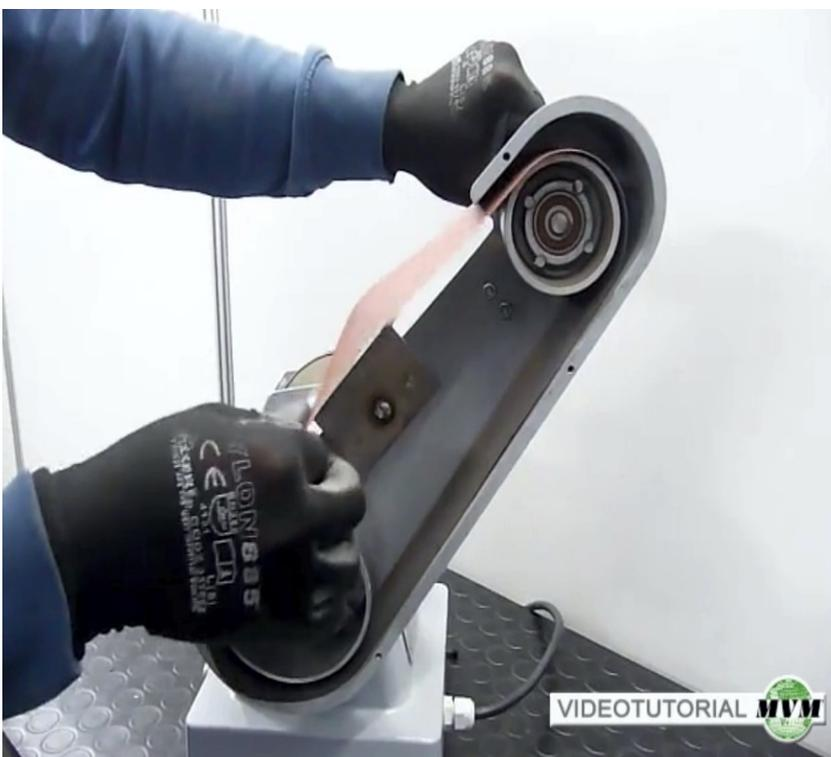
And remove the abrasive paper and then release the lever.
