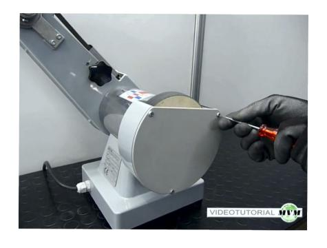
Remove the screws and remove the cover.
