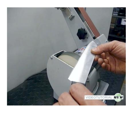
With a slight pressure pass the knife across the buffing wheel to polish the knife on both sides.
