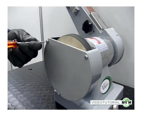
Finally, reposition the cover and tighten the screws.
