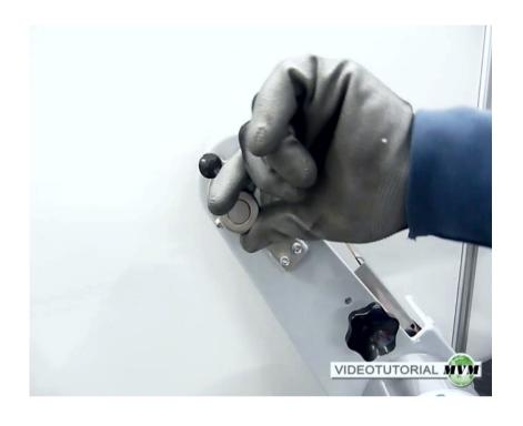
Turn the lever to loosen the belt.
