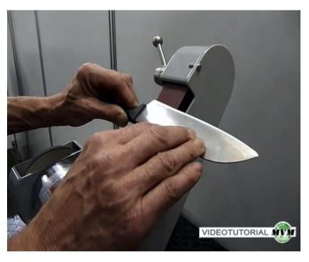
With a slight pressure pass the knife edge across the abrasive paper in the upper flexible zone to sharpen the bevel angle on both sides. The abrasive paper tends to adapt to the bevel angle of the knife.
