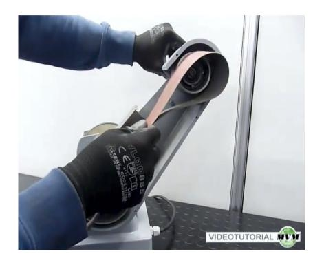
Turn the lever, insert the new abrasive paper band and then release the lever to tension the belt.
