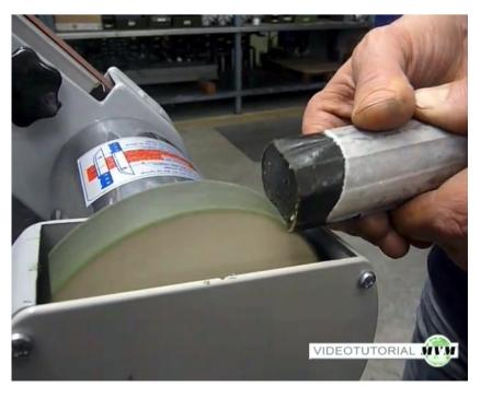
Apply silicone paste to the buffing wheel with a slight pressure of the stick of paste (supplied).
