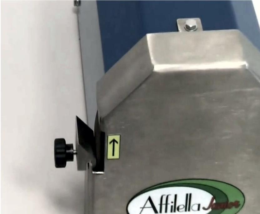
Fix the two 50 ° angle references on the grinding wheel housing, one on the right and one on the left of the grinding wheel.
