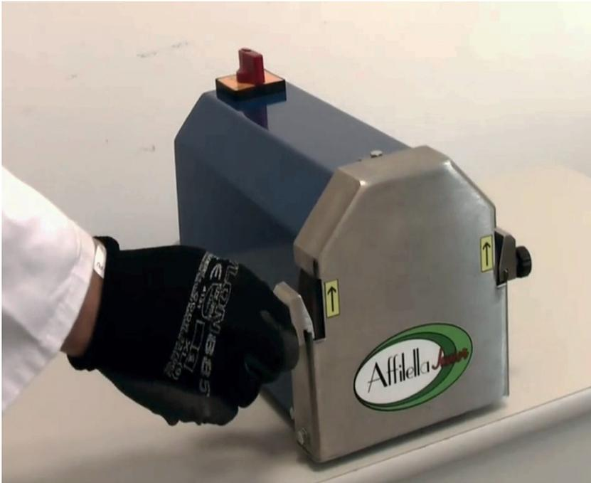
Fix the two 30 ° angle references on the grinding wheel housing, one on the right and one on the left of the grinding wheel.
