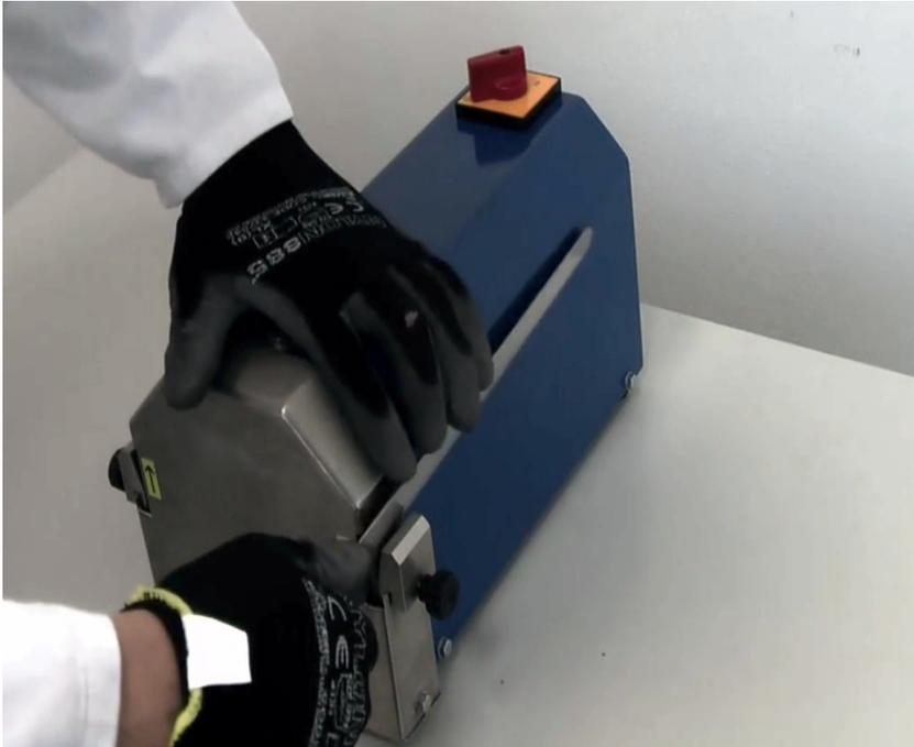
Turn the switch to position 2, place the blade of the knife on the right reference edge in contact with the grinding wheel and make 2-3 sharpening passes back and forth.
