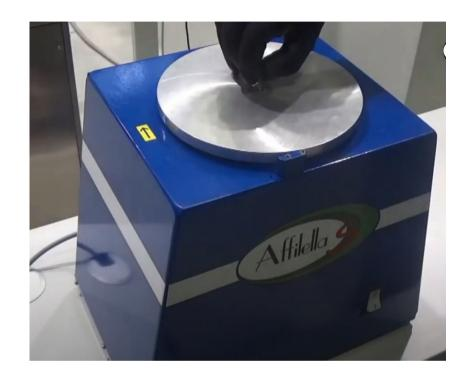
Place the aluminum rotating table and secure it with a M4X22 screw.
