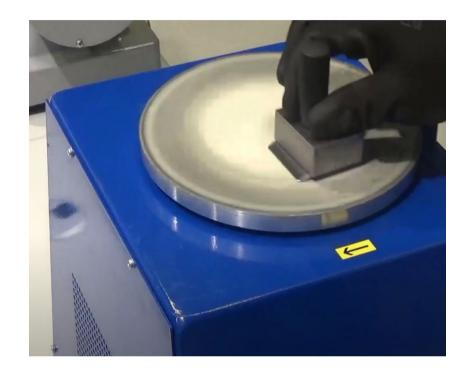
Manually bring the cutting head into contact with the rotating abrasive disc and press lightly.
