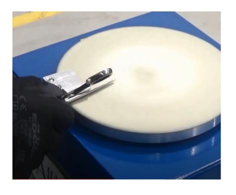
Place the inner blade of the scissors on the reference block angled at 40°, lean the blade slightly against the cloth and move the blade forwards and backwards slowly.
