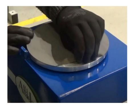
Remove the abrasive disk from the table.
