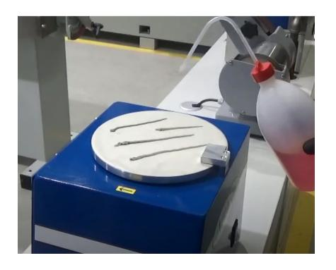
Dampen the cloth with alcohol to spread the diamond abrasive paste and manually spread the paste on the cloth.
