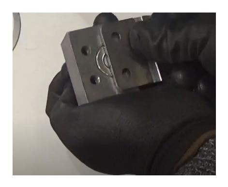
Mount the cutting head on the manual support holder.
