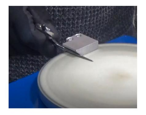
Pull the scissors out and repeat the same procedure with the other blade in the same way.
