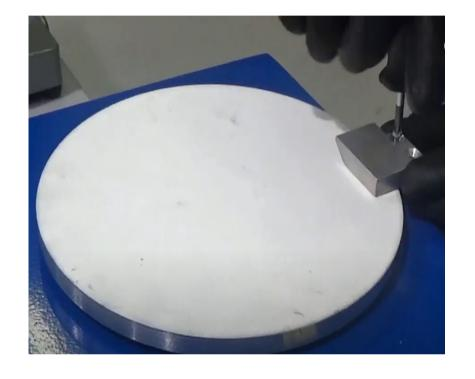
Secure the angled reference block (40°) in the proper support with the M4X12 screws.
