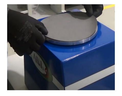
Place the adhesive abrasive disc carefully, ensuring that it perfectly adheres.
