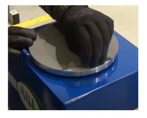
Remove the adhesive disc from the table.
