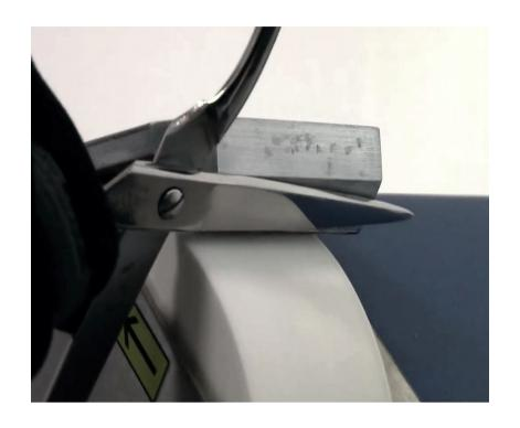
Place each blade of the scissors against the aligning reference tilted up at 45° in contact with the grinding wheel, then slide each blade 1-2 times across the grinding wheel.
