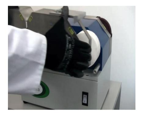
After replacing the wheels, replace the protective cover from the top, to its original position and tighten the 4 screws.
