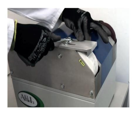
As the grinding wheel for sharpening scissors is consumed, you should adjust the reference alignment for the blade closer to the grinding wheel. Unscrew the 2 screws, manually adjust the position and retighten the 2 screws. Use a thickness of paper to check the distance between the reference and the grinding wheel.
