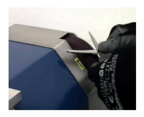
Pass each cutting edge of the scissors 1-2 times across the fabric buffing wheel to deburr and polish.
