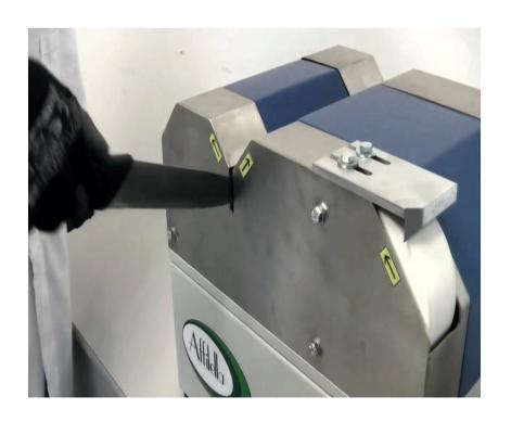
For knives with a curved tip end sharpen the blade by following the geometry of the cutting edge of the knife during the extraction from the grinding slot.
