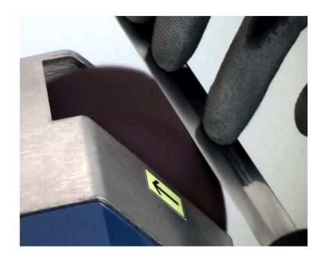
Pass the cutting edge 2-3 times for each side of the blade across the fabric buffing wheel for deburring and polishing.
