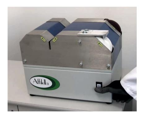
Plug the power cord into the power socket and switch on by pressing the on/off switch.
