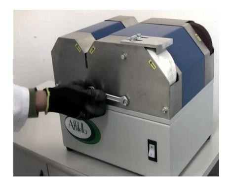
Unscrew the 4 screws on the upper protective wheel cover.
