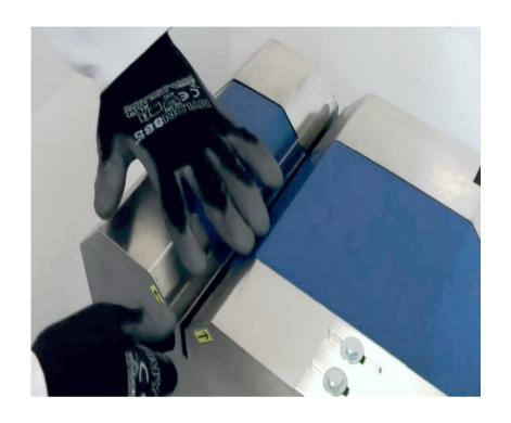
Insert the knife from above into the grinding slot until the blades makes contact with the grinding wheels, then slide the knife back and forth 2-3 times across the grinding wheels, finally extracting the blade from the front-side of the machine grinding slot.
