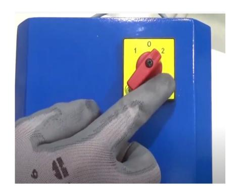
Turn the switch to position 1, to rotate the grinding wheel clockwise. Operate only on the left side of the machine.
