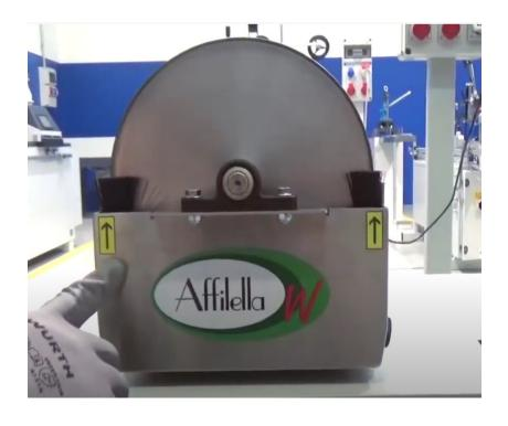
Turn the switch to 1, put the knife blade on the corner left reference block at 15° until it touches the grinding wheel, and pass the blade maximum 4 or 5 times.
