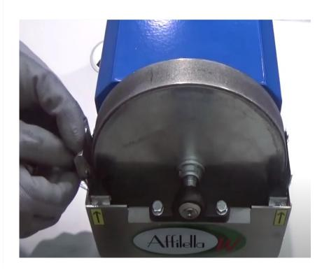
Place the 50° reference block on the edge grinding wheel cover, on the left side of the grinding wheel.
