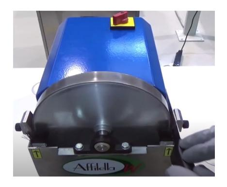
Turn the switch to 2, put the knife blade on the corner right reference block at 15° until it touches the grinding wheel, and pass the blade maximum 4 or 5 times.
