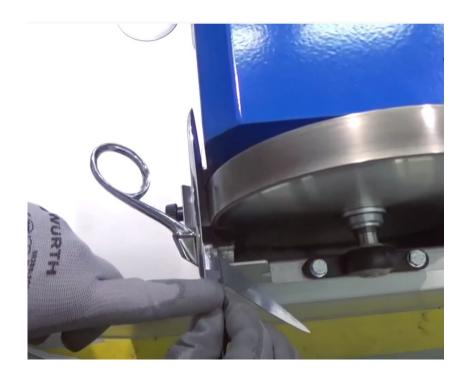
Turn the switch to 1, put the scissors blade against the reference block inclined at 50° until it touches the grinding wheel and pass each blade maximum 1 or 2 times.
